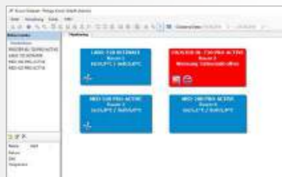
Monitoring overview of all integrated refrigerators and freezers. Malfunctions can be seen at a glance.
